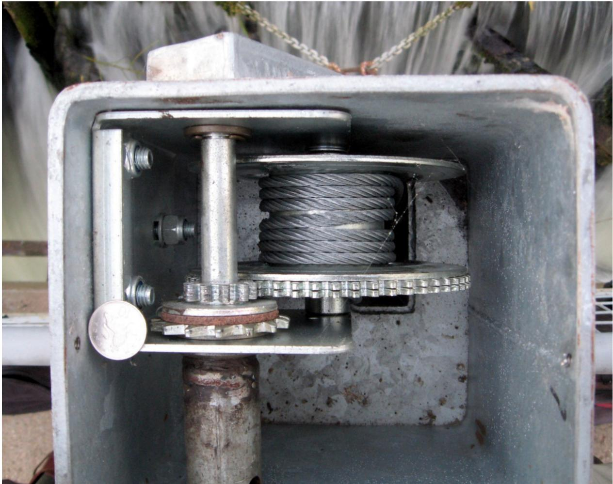
What weight does it have to lift? We have the 1961 drawings of the gate assembly. It is made of 3/16" thick steel, and the gates are 2' high by 7' wide. There are also the supporting arms. In the drawings the gates have a counterweight, but it was cut off when the manual winches were fitted a few years ago. With the steel frame and wooden base the gates work out at about 180 kg.
